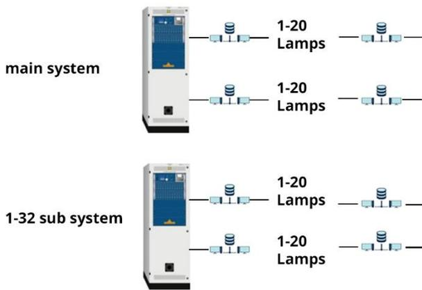
Figure 24: Systems networked via an external switch in connection with MC-BMS-EXT
