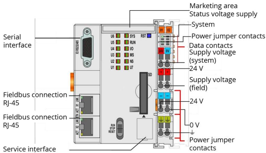
Figure 7: Connection diagram controller MC-BMS-EXT 750-821/00-100
