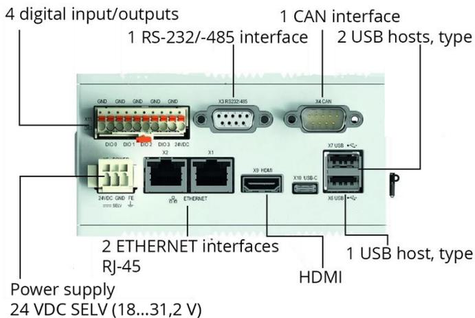
Figure 8: Connection diagramm controller MC-BMS 750-821/00-100
