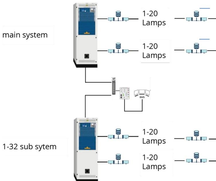
Figure 10: Networked systems connected to MC-BMS-EXT via an external switch
