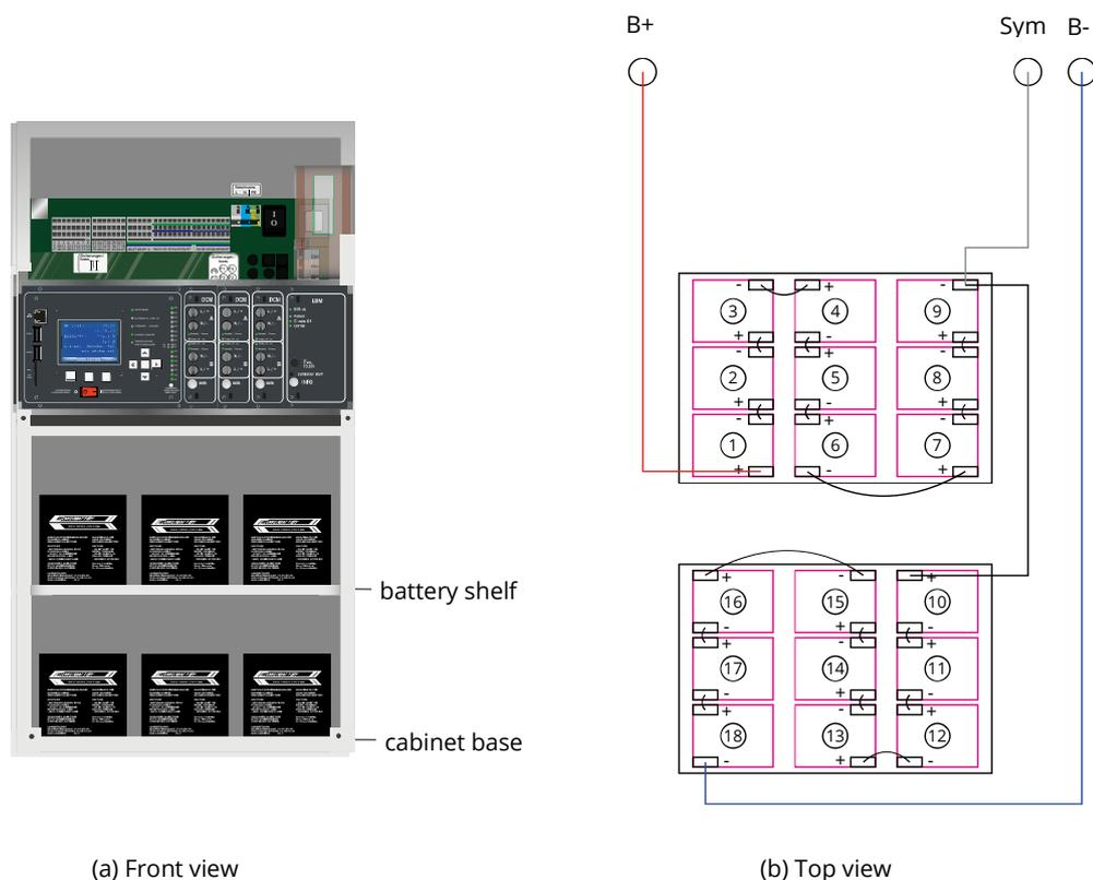
Figure 15: Mounting and connection of the battery blocks 12V 4.5Ah
