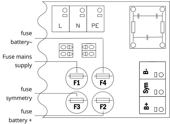
Figure 10: Fuses mains and battery supply
