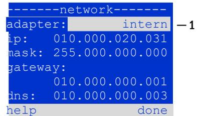
Figure 59: submenu for setting ip-addresses
