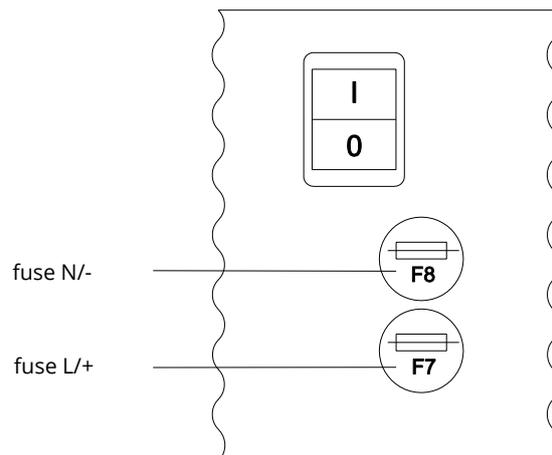
Figure 7: Fuse auxiliary circuit
