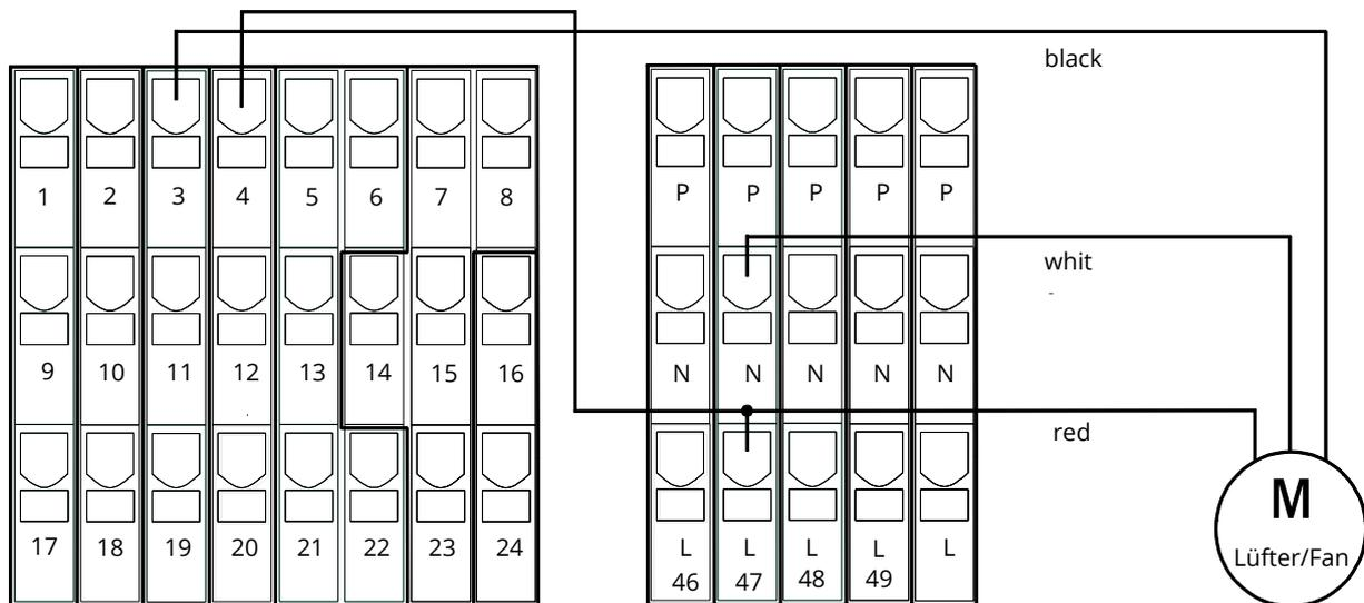
Figure 14: Connection terminals for an internal fan
