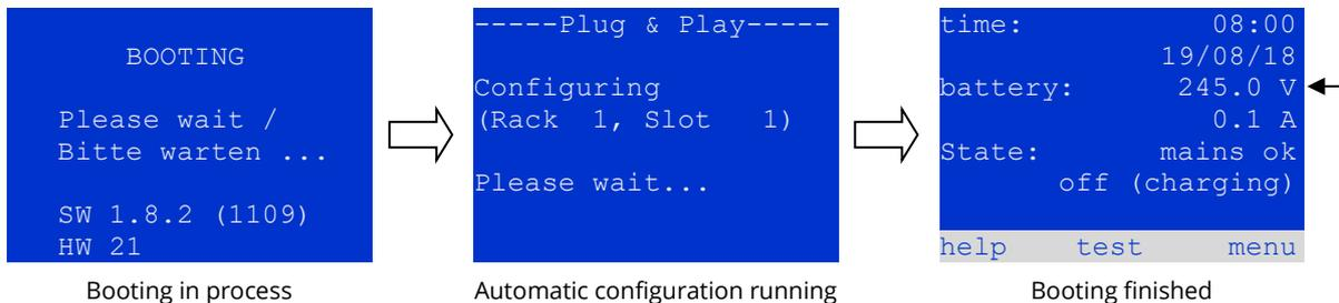
Figure 20: Boot process (left, middle) and status message (right).
