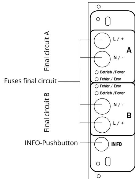
Figure 17: DCM-circuit module
