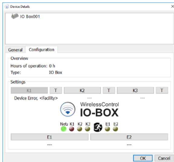
Figure 91: Device Details window for IO boxes, Configuration view
