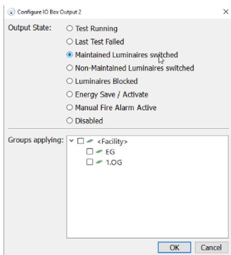
Figure 92: Configuring the IO box output
