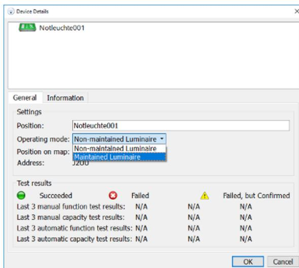
Figure 88: Device details window for emergency luminaire operating mode
