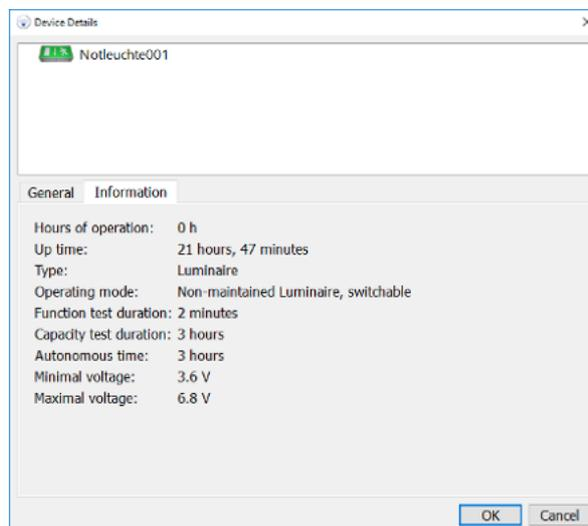
Figure 87 Device details window for emergency luminaire Information tab
