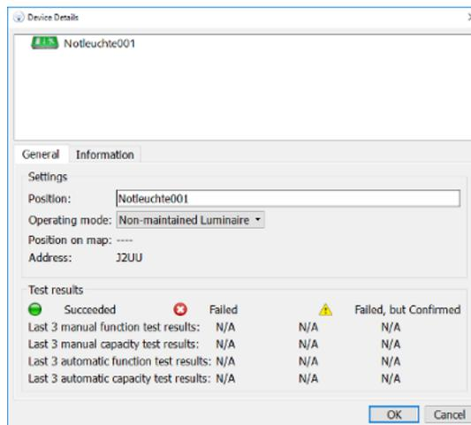
Figure 86 Device details window for emergency luminaire General tab
