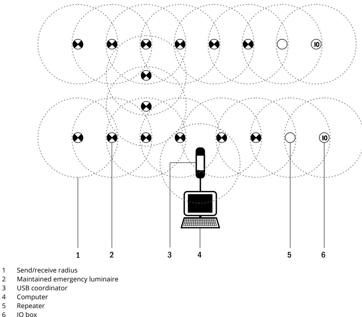
Figure 7: Setup of a WirelessProfessional system
