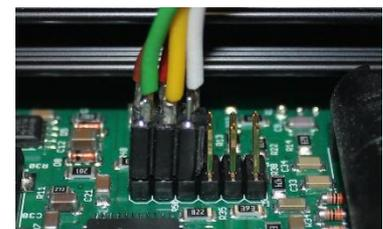
Figure 4: Position of programming connector
