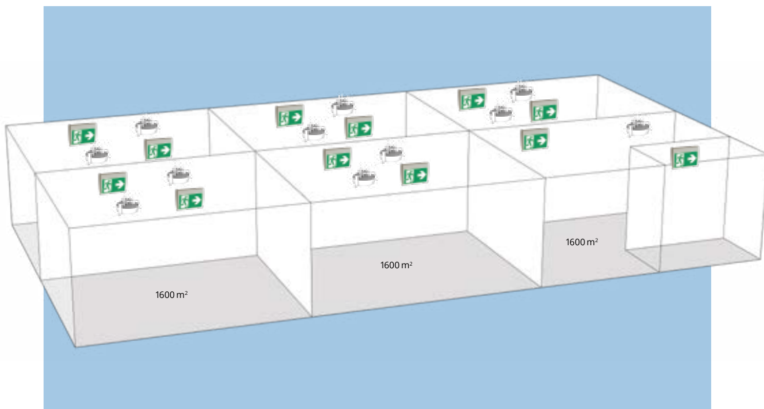
Example of a restaurant with virtual fire compartments
