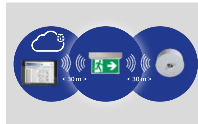
Wireless luminaire monitoring and control with Wireless Professional
