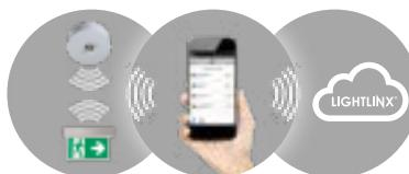
All data of your installation will be saved in the RP-Cloud (after a one-time registration). Details on the status or configuration can be called up there at any time. Lightlnx® enables secure access to all data and an overall visualization of all your installations via an Internet browser. The clear one Depiction of the
