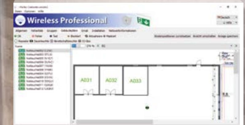
In addition or as an alternative, the WP software can also be used on our compact Wireless Embedded PC or an existing Windows system. You can then set up and visualise your emergency lighting system from the comfort of your office. The system monitors the luminaires and reduces the amount of maintenance work needed.
