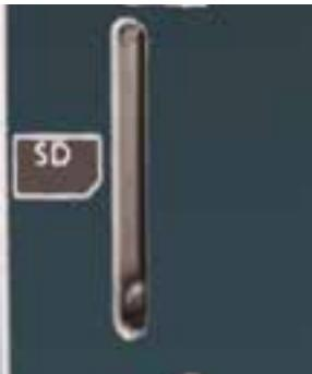
The software of the NLSR is continuously developed. With the integrated interfaces (SD card slot, USB ports), it is possible to load new firmware without any special programming knowledge.
