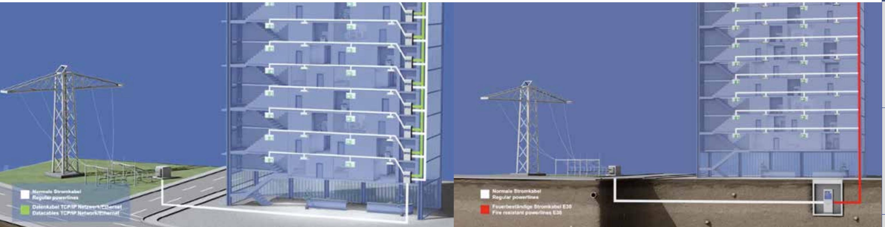
Power supply systems with limited output (Low power systems) form the concept of decentralization of fire compartment-related safety lighting systems to supply emergency and safety lights in the fire compartment. This decentralized concept makes the use of cables in the maintenance of functions, for supplying the lights, superfluous according to MLAR 2005.
