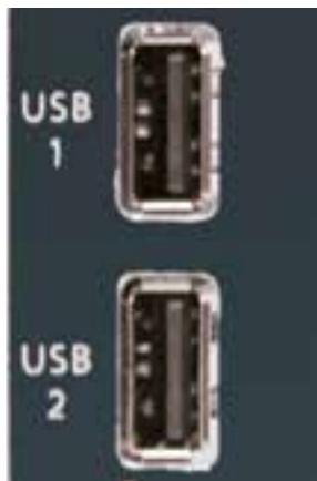
The integrated USB ports offer the option of a standard USB keyboard for configuration of the system via LCD, connection of an external printer (PCL6) and firmware update using a USB stick.
