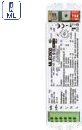
The **MLED500** is an electronic switching power supply with integrated individual light monitoring, light management function, mains monitoring, dimmer and flashing functions. All switching modes are possible. The mains monitor allows the operation of connected luminaires in non-maintained mode in a maintained circuit. In case of a mains failure all lights are switched on automatically. LED illuminants with a max. output of 8W can be used as consumers.
