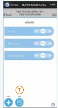
*Troubleshooting: If there are no installed luminaires in the luminaire list, please check your network. Is the title line showing "Network connected"? If not, tap on "Connect". Once the connection has been established, you can reload the luminaire list by tapping on "Update".*
