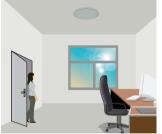
With sufficient natural light, the light does not switch on when presence is detected.
