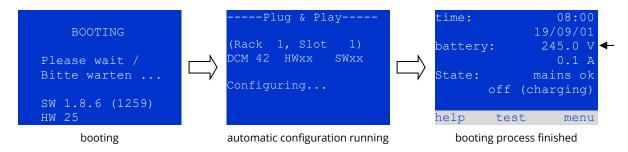
Figure 3: Booting process (left, centre) and status (right)
