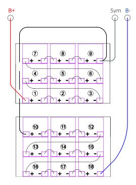
Figure 2: Wiring of the batteries top view
