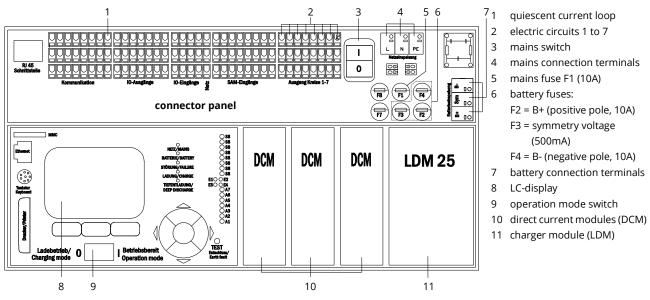
Figure 1: View of the opened microControl plus system
