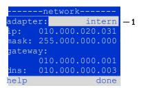
Figure 59: submenu for setting ip-addresses
