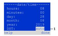
Figure 67: Setting the system time
