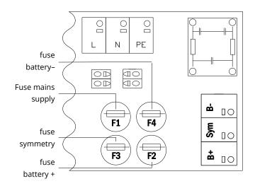
Figure 10: Fuses mains and battery supply
