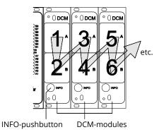
Figure 22: Numbering of the circuits
