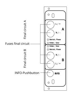
Figure 17: DCM-circuit module
