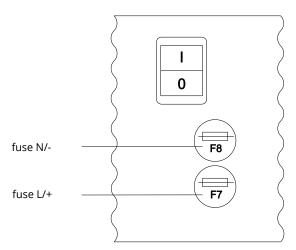
Figure 7: Fuse auxilliary circuit
