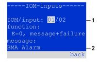
Figure 63: Programming of the IOMinputs
