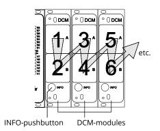
Figure 18: Numbering of the circuits
