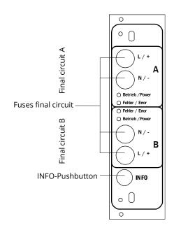
Figure 14: DCM-circuit module
