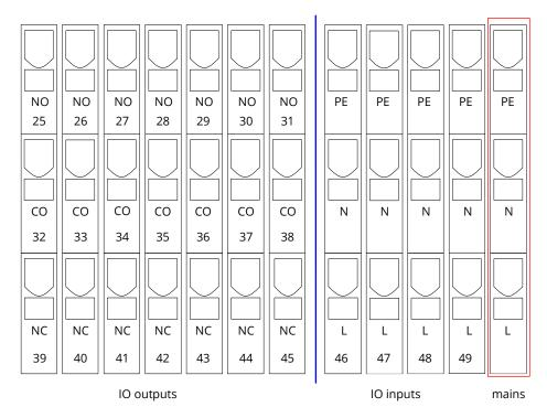
Figure 4: In- and outputs IO-module
