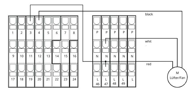
Figure 11: Connection of a fan
