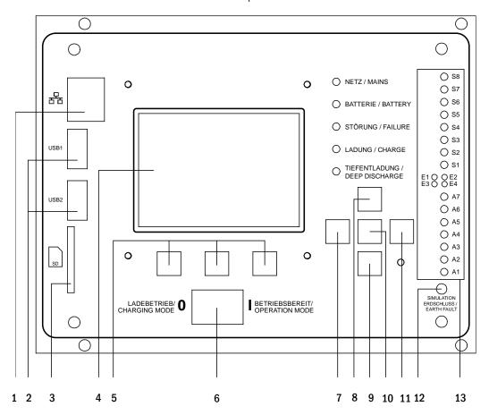
Figure 13: Central control and monitoring unit
