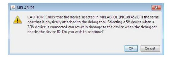
If this error message also appears during other process steps, it does not indicate a faulty operation. Just click on OK then.
