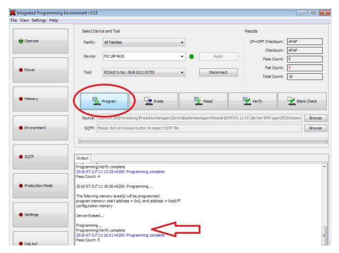
The written data are automatically checked after the programming. The successful completion of the programming is indicated by the line *Programming/Verify complete* or *Programming complete*.
