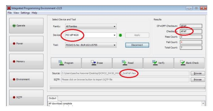
If the PICkit3 is already connected to the PC, it is shown in the field *Tool*. Otherwise connect it now. Then select the PICkit3 by clicking on *Connect*. If the following error message appears, click on *OK*:
