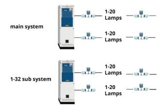
Figure 24: Systems networked via an external switch in connection with MC-BMS-EXT
