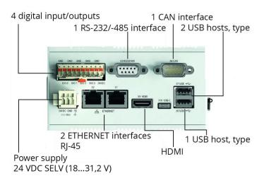
Figure 8: Connection diagramm controller MC-BMS 750-821/00-100
