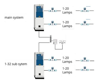
Figure 10: Networked systems connected to MC-BMS-EXT via an external switch
