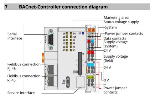
Figure 7: Connection diagram controller MC-BMS-EXT 750-821/00-100
