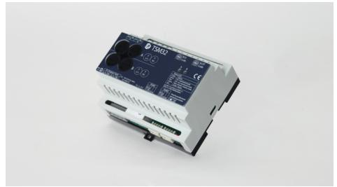
Thanks to integrated individual luminaire query, self-calibrating circuit monitoring and earth fault and fault voltage monitoring (when the circuit is not active), the modules ensure maximum operational reliability. All relevant status data can be conveniently retrieved at any time on the central computer via the integrated INFO button.
