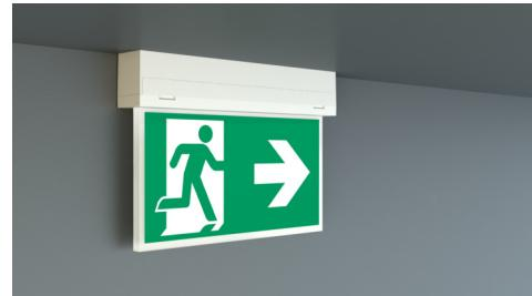
Thanks to the snap-in mechanism between the upper and lower part, the luminaire has a harmonious look and appears closed all the way round. The luminaire is connected to the mains in the ceiling section. When closed, the luminaire is powered via contact plugs. This greatly simplifies mounting and makes convenient connection possible despite the small size of the luminaire.
