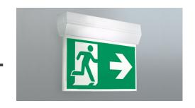
Planning certainty is provided by tool-free, variable use of the pictograms on site. A set of pictograms corresponding to DIN ISO 7010 (arrow to the right, left, up and down) is supplied as standard. Universal mounting includes fitting on the wall and ceiling as well as the option of fitting in the ceiling in conjunction with the mounting frame available.
