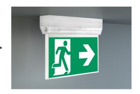
Control and monitoring via central power supply system. Planning certainty is provided by tool-free, variable use of the pictograms on site. A set of pictograms corresponding to DIN ISO 7010 (arrow to the right, left, up and down) is supplied as standard. Universal mounting includes fitting on the wall and ceiling as well as the option of fitting in the ceiling in conjunction with the mounting frame available.
