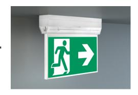
Automatic monitoring of safety luminaire with SelfControl. Planning certainty is provided by tool-free, variable use of the pictograms on site. A set of pictograms corresponding to DIN ISO 7010 (arrow to the right, left, up and down) is supplied as standard. Universal mounting includes fitting on the wall and ceiling as well as the option of fitting in the ceiling in conjunction with the mounting frame available.
