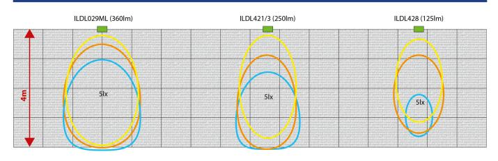
Abstand zur Wand / Distance to wall 1m Abstand zur Wand / Distance to wall 1,5m Abstand zur Wand / Distance to wall 2m
