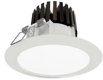
LED recessed and surface-mounted downlight, RAVIO series. IP20 (for the surface-mounted version). Housing made from plastic (PC) and passive aluminium cooler. Diffuser made from plastic, opal. Operating unit can be switched or dimmed (DALI dimmer), external (integrated in the surface-mounted version). Version with Casambi Bluetooth control available. DC compatibility on request.
