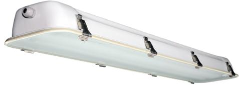
LED moisture-proof luminaire, LUKA series, IP66. Resistant to ammonia and oil. Housing made from steel plate. Diffuser made from safety glass. Feed-through wiring present. Power supply, can be switched or dimmed (DALI dimmer), integrated. DC compatibility and NANO protection on request. Suitable for use in the food industry. Area of application: car washes, chemical industry, kitchens etc.
