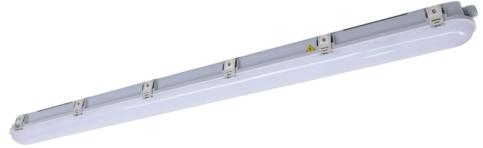
LED diffuser luminaire, VASCA series, IP65, IK08. Housing made from polycarbonate. Prismatic diffuser made from PC, UV-resistant. Diffuser is fastened with stainless steel clips. LED boards can be interchanged individually. Operating unit (DALI dimmable), installed. Feed-through wiring present. Version with Casambi Bluetooth control available. DC compatible.
