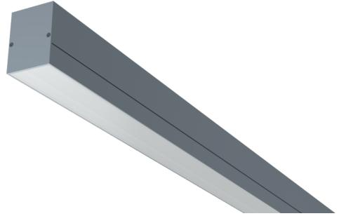
LED ceiling- and wall-mounted luminaire, MAVS. Housing made from aluminium, white, powder-coated. Diffuser made from plastic (PMMA), opal, UV-stabilised. Operating unit can be switched or dimmed (DALI dimmer), integrated. Version with
