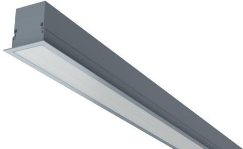
LED ceiling- and wall-mounted luminaire, MAVS. Housing made from aluminium, white, powder-coated. Diffuser made from plastic (PMMA), opal, UV-stabilised. Operating unit can be switched or dimmed (DALI dimmer), integrated. Version with
