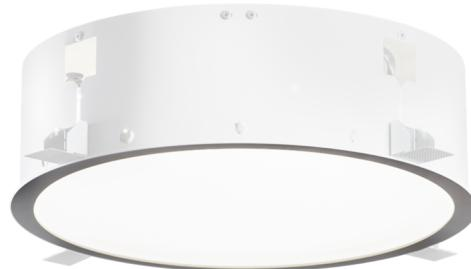
LED ceiling- and wall-mounted luminaire, PORIO series, recessed design, as the basic lighting for commercial and residential rooms. Housing made from steel plate, white, powder-coated. Diffuser made from plastic (PMMA), opal, UV-stabilised. Operating unit can be switched or dimmed (DALI dimmer), integrated. Version with CASAMBI Bluetooth control available. DC compatible.
